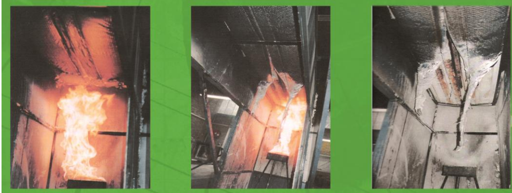
C. Flexible Foil faced Fibre Insulation – Material above fire source destroyed but no ignition whatsoever.
