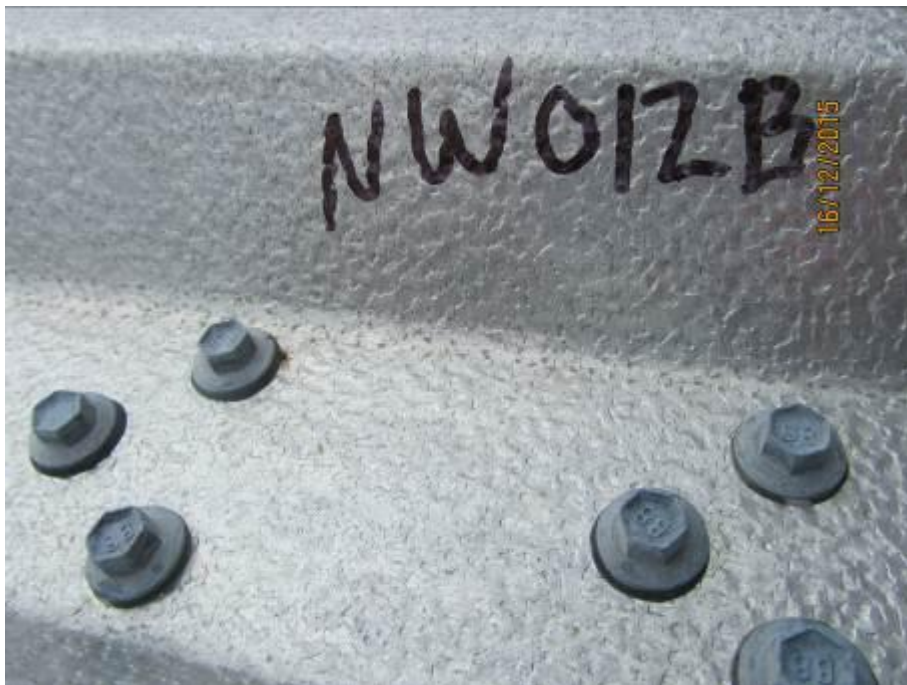
Photograph No3 Exceeded Class 4 for AS 3566.2.
