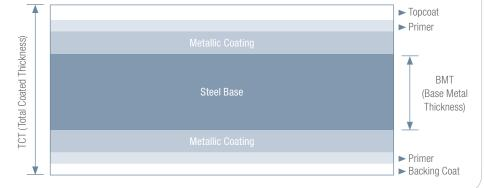
It is important to note that structural capability is a function of BMT and steel grade whereas corrosion performance is afforded by metallic coating thickness and type. Always ensure that the BMT specified is as per recommendations.
