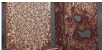
Galvanised steel: Washed panels - Exposed for 12 years
