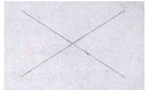
ZINCALUME® steel @ 240 hours of salt spray testing.
